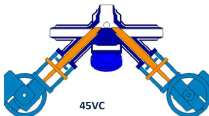
SchuF can deliver diverter valves in both designs with up to seven inlets and outlets. The type 45VC shown here has one inlet and four outlets, in this case each outlet is separately controlled with a contoured piston and an electric position control actuator.
